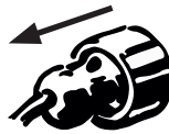
During inspection and maintenance, servicing and removal of trapped waste. Disconnect the power to the machine by removing the plug from the wall socket.
